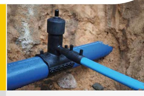
The newly developed AGRU pressure tapping valve (DAV) creates re-closable branches on existing PE pipes. A fast, simple and safe installation is possible when using a pressure tapping valve. The installation and tapping can be performed during the operation under full working pressure. The pressure tapping saddle consists of premium materials, which ensures an absolute reliability and a complete maintenance-free operation.
