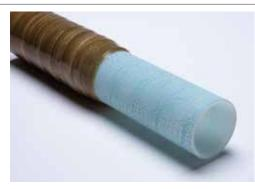
The PVDF HV-Liner from AGRU is an economical alternative to traditional fabric backed pipes. The surface-treated PVDF pipe has a three-dimensional surface structure that provides an optimal bonding to the FRP pipe. The piping systems are available in PVDF, PVDF-FLEX, and PVDF-el. The pipes can be produced in diameters from 20 – 400 mm.
